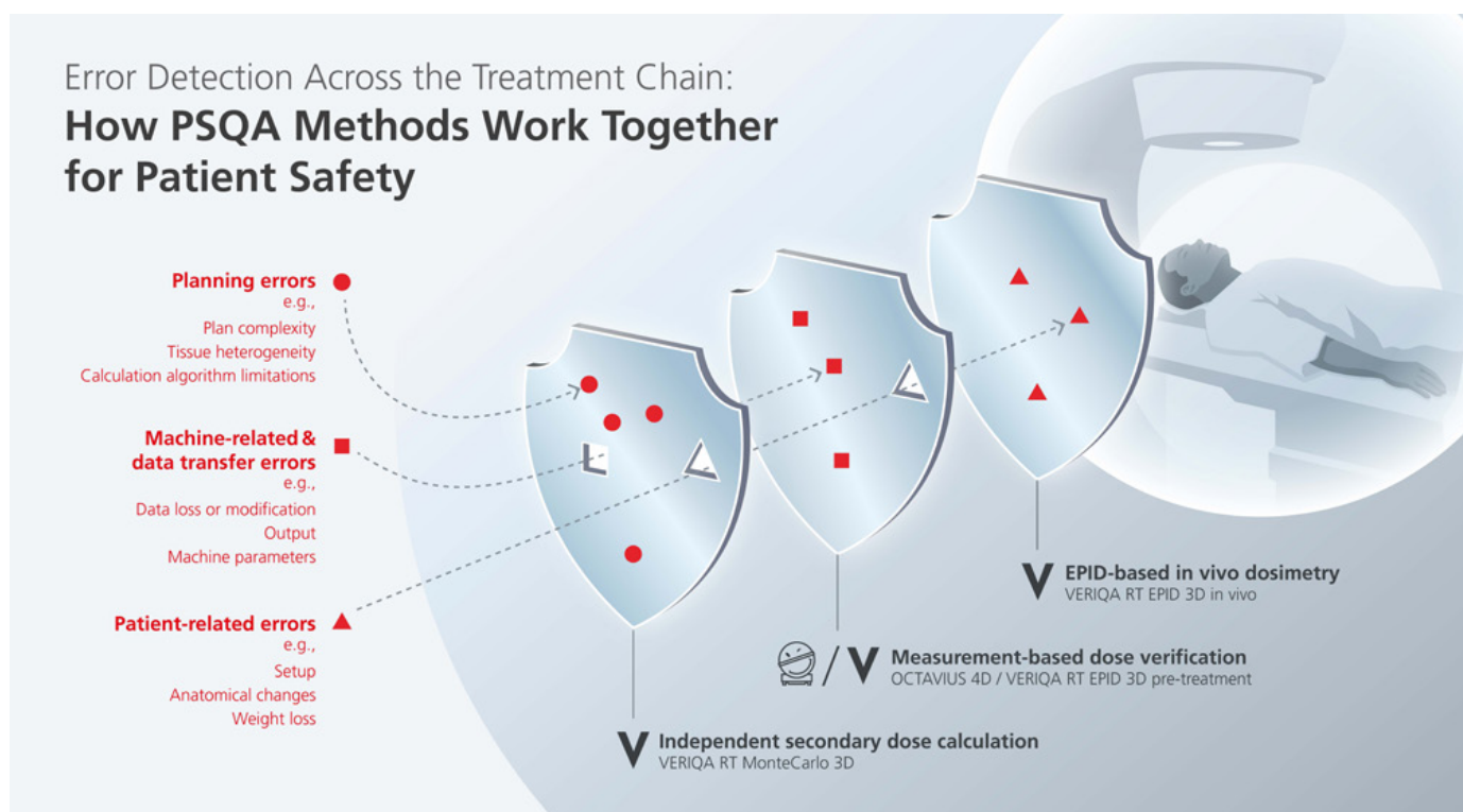
Figure 1. Different PSQA methods address different error sources. Independent dose recalculation, EPID dosimetry, and phantom-based measurements provide complementary verification of planning, transfer-related, machine-related, and patient-specific errors.
